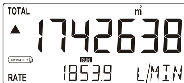
Fig. 4: Example of low-battery alarm.
