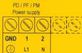
The GND terminal shall be connected to a Functional Earth (FE), the L1 lead shall be connected to terminal 1 (internally fused) and the Neutral lead shall be connected to terminal 2.
